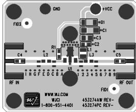
Circuit Board Material: .014" Getek, 4 layers (other layers added for rigidity), .062" total thickness, 1 oz copper Microstrip line details: width = .026", spacing = .026"
